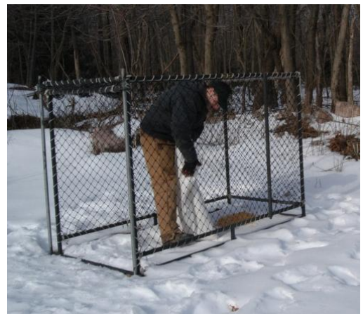
A Clover trap baited with corn. Deer enter to eat the corn, hit a trip wire, and a net door falls down to capture them in the trap.
